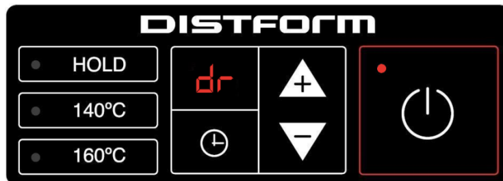
Figure 4. Control panel for model without humidity system when the door is open
